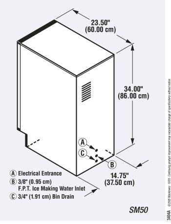
Installation Note - There is no minimum clearance required, designed to be integrated into cabinet opening 15.00" (38.00 cm) wide.
